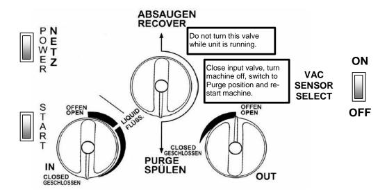
**NOTE:** To change from Recovery mode to Purge: Close the Input port, turn the unit off (to prevent high pressure shutoff), switch to Purge position and restart the unit.
