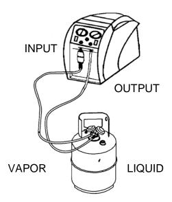
To start you must have a minimum of 2,5 kg of liquid refrigerant in the tank.
